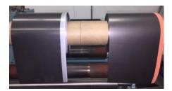
**Figure 2.** Dry battery electrode NMC roll (left) and graphite roll (right) double sided laminated onto current collector which is ready for cell assembly.
